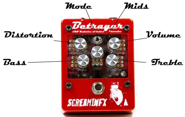
*Pedal labels are etched on the top clear abrasion resistant layer and drawn on the circuit board below.*
