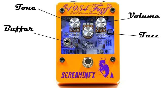
*Pedal labels are etched on the top clear abrasion resistant layer and drawn on the circuit board below.*
